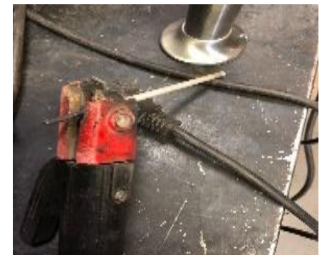
Figure 8. Damaged welding tongs Source: Author's own work.
