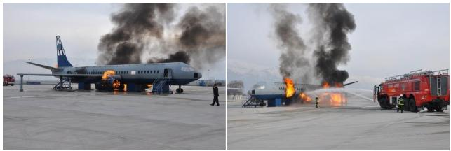
Aircraft Fire Fighting Simulator simulates Boeing 737-800 type aircraft with exact measurements. It is possible to start a live fire in 28 different sections inside and outside the aircraft, meeting all the intervention methods prescribed by ICAO.
