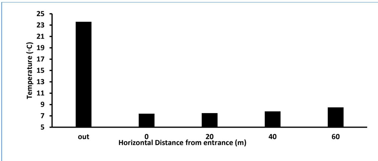
Figure 9 Temperatures at Different Locations of the Mantar Cave
