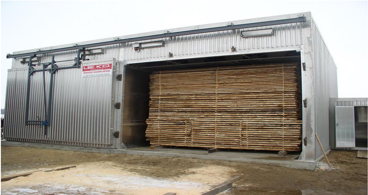
Figure 6. The wood KD or Kiln Dryer, used to dry wood lumbers to wanted humidity
