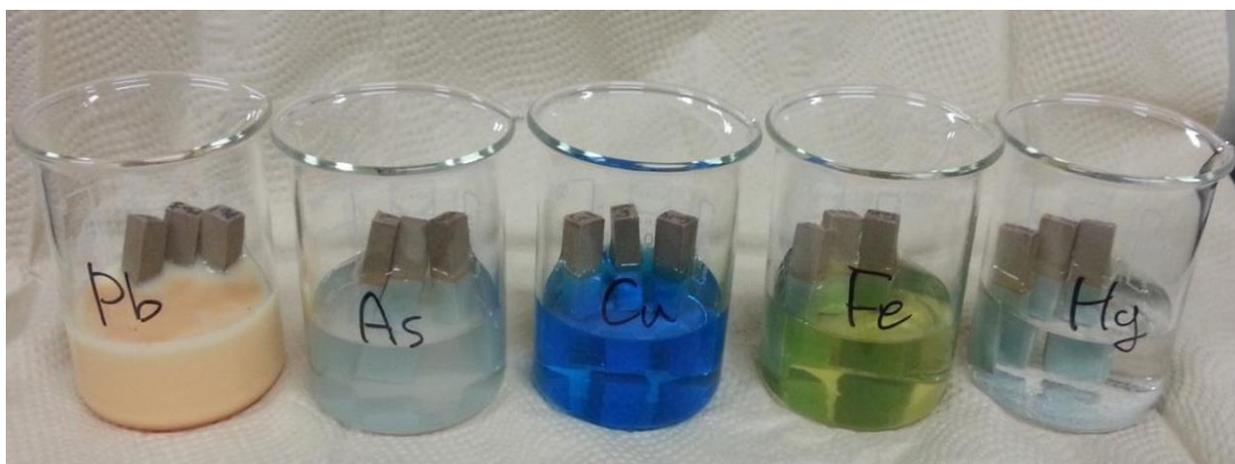
**Fig.4.** Celadon samples immersed in the test solutions.
